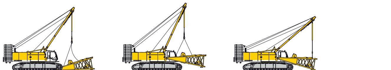
Unloading and assembly of boom foot
